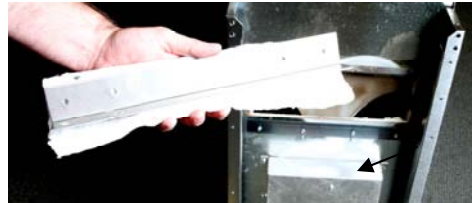
Figure 2: Position the bracket on top of the insulating material and press the material into place atop the box behind the burner chamber. See arrow and drawing below.
