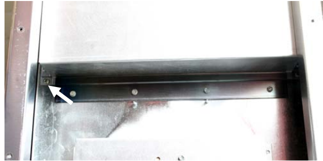
Figure 1: Four screws and a bracket secure the flue to the rear of the fryer. An extension will be needed to reach the screws. See arrow.
